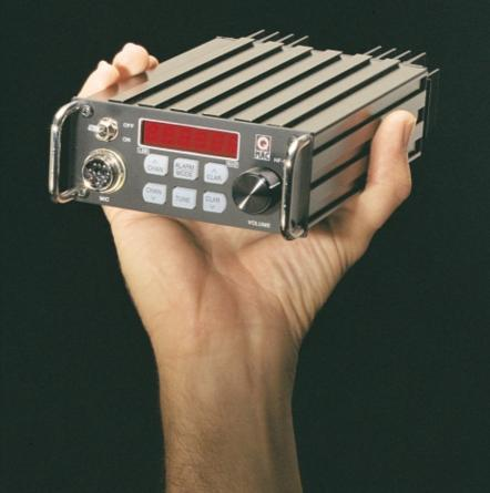
The HF-90 is a rugged all-purpose HF SSB transceiver, designed for man-pack, portable, vehicle and fixed base station applications. It is an extremely compact and light weight unit, featuring only essential controls to ensure ease of operation.
